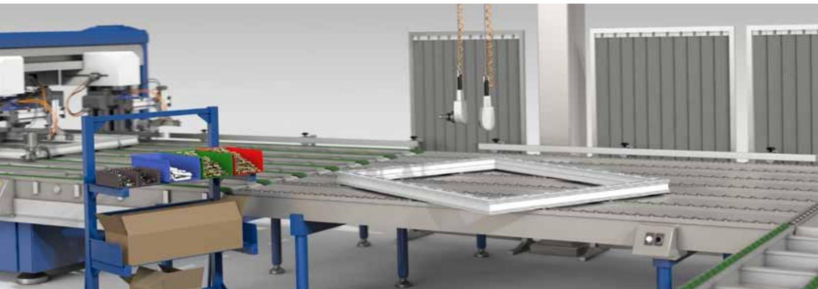
The essential tasks of automatic installation of fittings are drilling and bolting components of all kinds, e.g. fittings and reinforcements.
