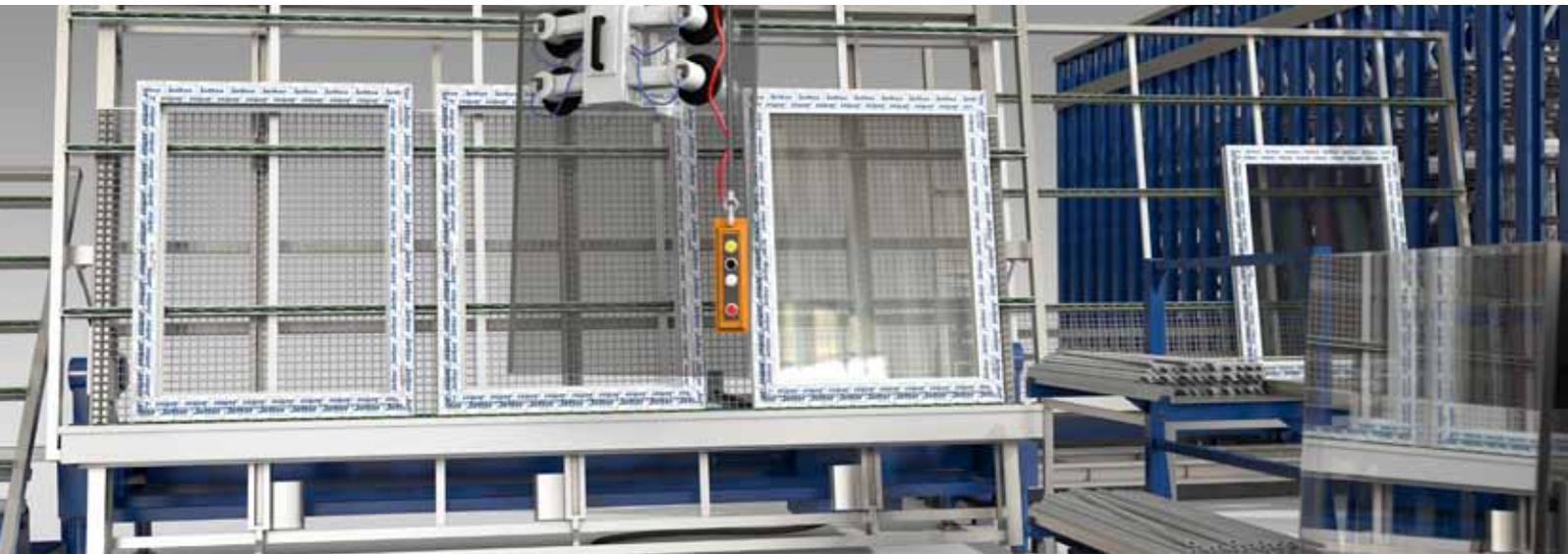
The logistical challenges for glass panels are especially high. Along with enormous transport weights and different formats, it must be possible to store and transport the material safely without any damage. Window and glass elements are then joined in an automated process.
