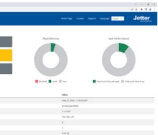
JetSym also offers a toolbox of functions for fast diagnostics and response to more complex faults. Triggered by freely definable limit values, log data are automatically recorded in the controller, or an oscilloscope recording is started. This can be imported and analyzed in JetSym by service technicians at a later time.
