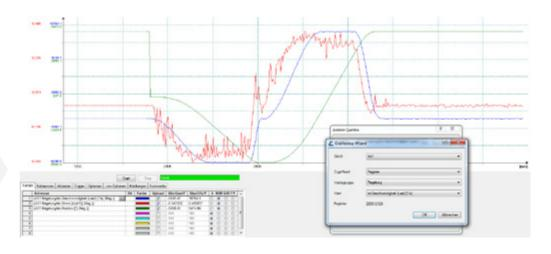
JetSym provides programmers with effective tools for the precise analysis of the program flow. The integrated debugger can be used to step through the code and to display the values stored in variables. The trace and monitor function allows values to be monitored during the program flow without having to interrupt the actual program.
