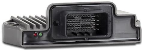
Communication with the JXM-IO-E30 takes place via CANopen®. This allows for integration into conventional CAN networks used in mobile machinery.
