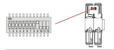
Position of the DIP switch sliders at the JX3-BN-ETH and JX3-COM-EIPA/-PND
