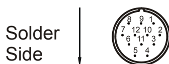
Fig. 31: View on RC series mating connector of the EnDat (internal thread M23)
