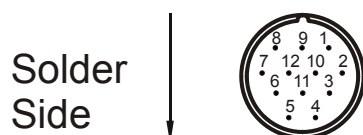
Fig. 12: View on the RC series mating connector of the resolver (internal thread M23)
