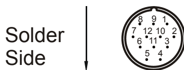
Fig.: 19: RC series mating connector of the EnDat (internal thread M23)
