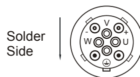
Fig. 11: View on the SM series mating connector of the motor (internal thread M40)
