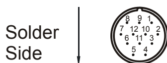
Fig. 12: View on the RC series mating connector of the resolver (internal thread M23)
