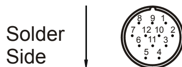
Fig.: 28: View on RC series mating connector of the EnDat (internal thread M23)
