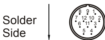
Fig.: 11: RC series mating connector of the resolver (internal thread M23)
