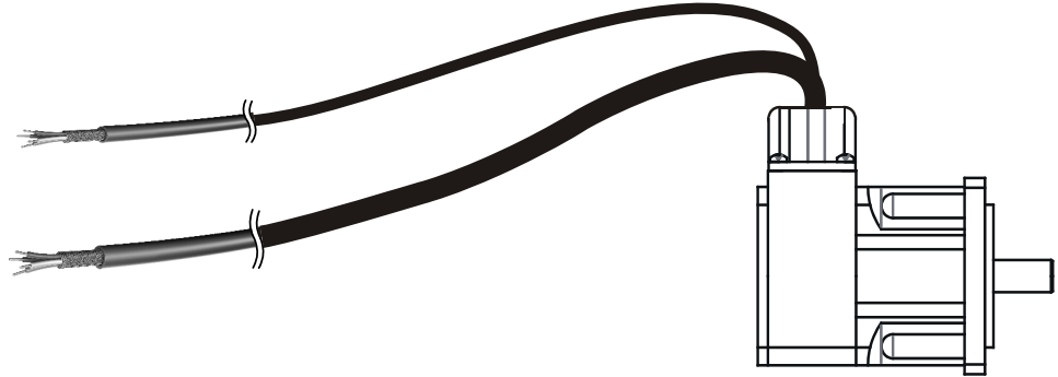
Fig. 14: Motor with cable and without a male connector
