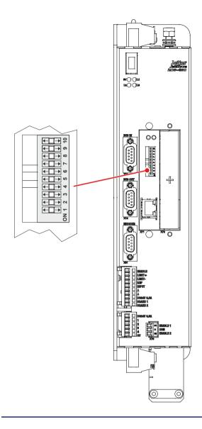
Assigning the IP address and the GNN to the JX3-BN-ETH and JX3-COM-EIPA/-PND
