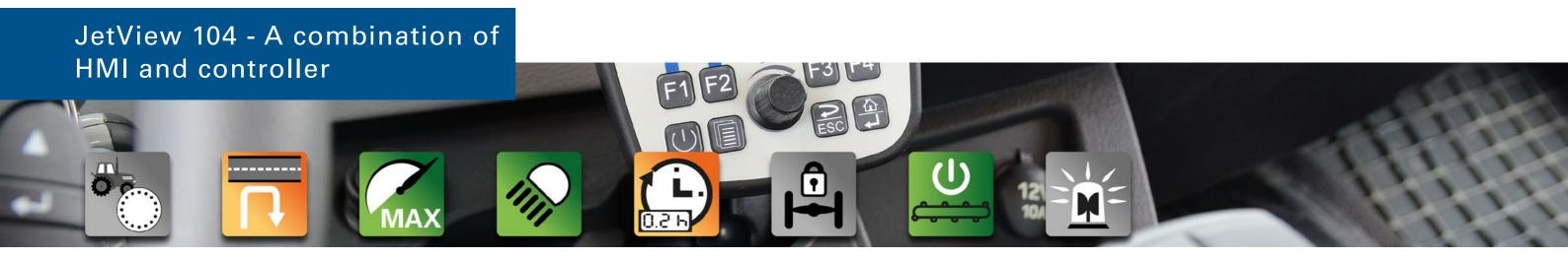
The JetViewMobile 104 is a very compact combination of a smallsize HMI and an integrated high-performance controller. The JVM-104 is available in various configuration levels. From the basic version with a simple CANopen interface to the full version with two CAN interfaces, RS232, USB and M12x1 Ethernet port, the display controller can be ideally adapted to any task.
