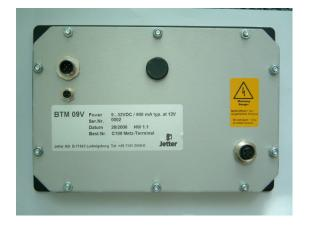
On the rear of the device there are 3 waterproof plugs/sockets and the venting element to equalize pressure.
