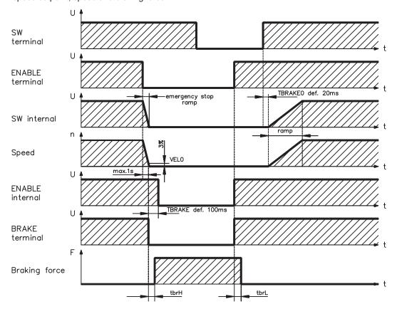
During the internal ENABLE delay time of 100ms the speed setpoint of the servo amplifier is internally driven down a 10ms ramp to 0V. The brake output is switched on when 3% of the final speed is reached.
