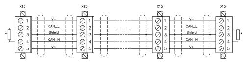
\* according to line impedance about  $120\,\Omega$
