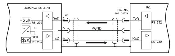
Interface cable between the PC and servo amplifiers of the JetMove 640/670 series:
