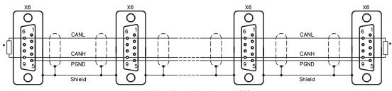
\* according to line impedance about  $120\,\Omega$
