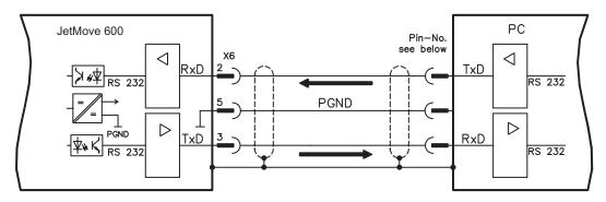
Interface cable between the PC and servo amplifiers of the JetMove 600 series:
