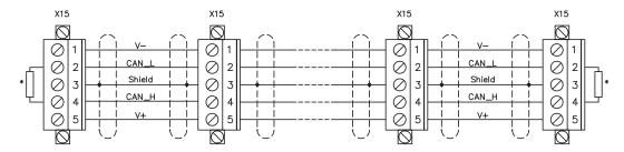
\* according to line impedance about  $120\Omega$
