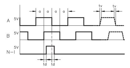
Edge spacing a  $\geq$  0,20  $\mu s$ Edge steepness tv  $\leq$  0.1  $\mu s$ Delay N-I-td  $\leq$  0.1  $\mu s$  $|\Delta U| \geq 2V/20 mA$
