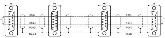
\* according to line impedance about  $120\Omega$
