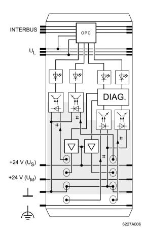
Figure 3 Internal wiring of the terminal points
