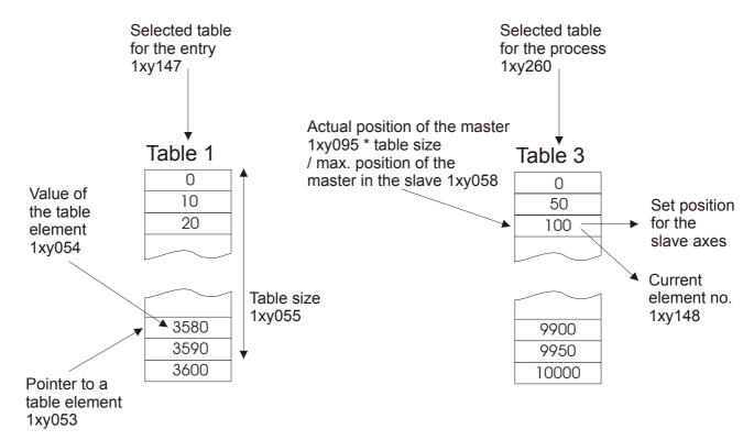
As in previous versions, different table sizes are allowed. As long as register 1xy260 is not written, register 1xy147 is used as selected table for the process.
