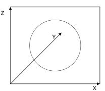
Case 3: Circle in the y-z level. Rotated  $90^\circ$  around the y-axis. 1z4087=0 1z4088=90000 corresponds to  $90^\circ$  1z4089=0
