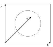
Case 3: Circle in the y-z level. Rotated 90° around the y-axis. 1z4087=0 1z4088=90000 corresponds to 90° 1z4089=0
