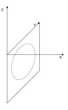
Case 4: Circle in the x-y level. Rotated 90° around the z-axis. 1z4087=0 1z4088=0 1z4089=90000 corresponds to 90°
