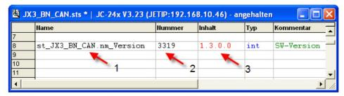
Figure 3: SW version, displayed in the format of the IP address
