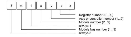
The module bus number "m" designates the number of the module bus position on the CPU.
