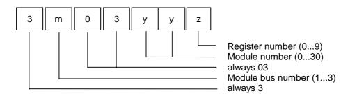
The module bus number "m" designates the number of the module bus position on the CPU.
